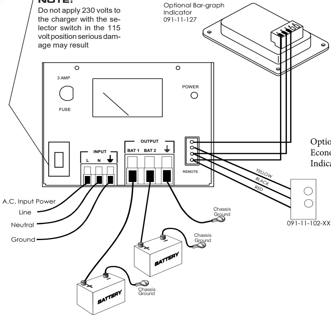
**IMPORTANT:** Charger output wire size is 14 awg. Wire size is for a maximum length of 20 feet. If wiring is to be longer, larger wiring is required. Additional information is available on request.
